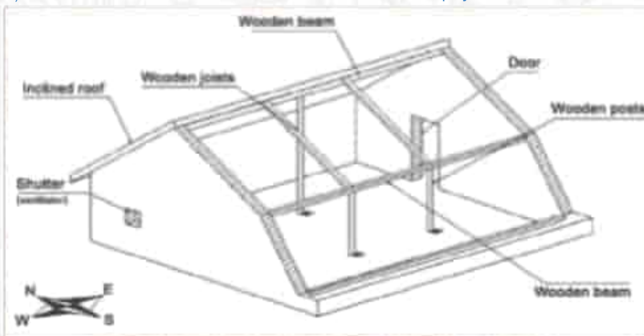
Picture No. 13: Schema of the wooden structure for the polythene sheet fixation
