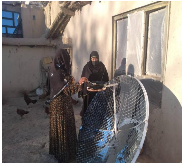
Figure 3: Cooking with a solar cooker.
