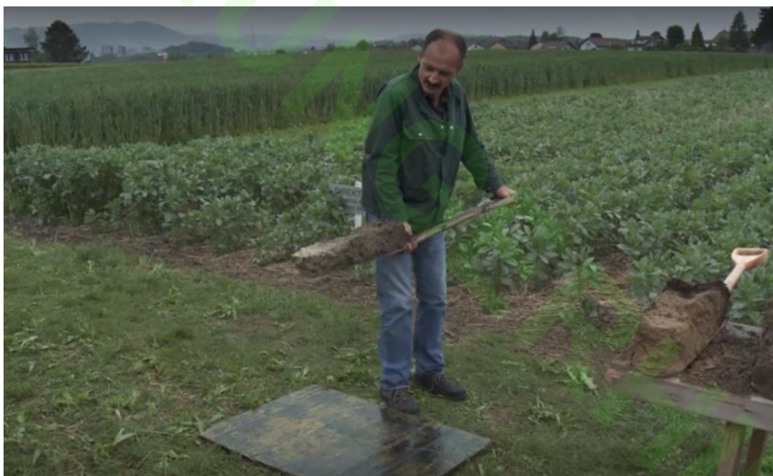
Dropping the soil from a spade onto a plastic board (spade shatter test).
