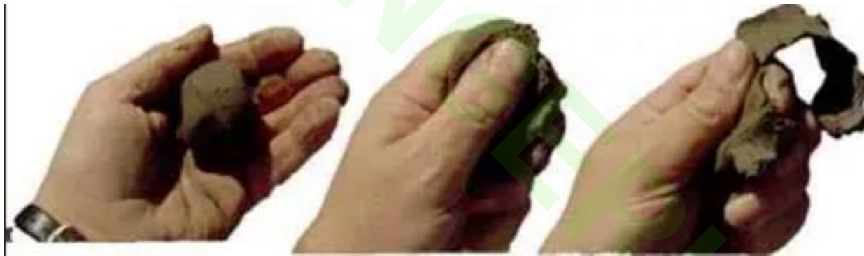
Making a ball from soil and pressing the ball to feel its texture.
