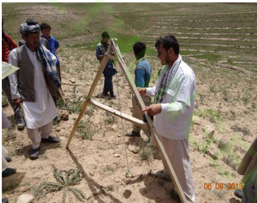
Figure 16: The A-frame can be used for making terraces and leveling.
